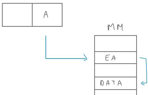
The address field A in the instruction does not contain the actual data's memory location. Instead, A holds a memory address where the **effective address (EA)** is stored. The processor first retrieves the EA from this memory location, then uses it to access the actual data in main memory.
