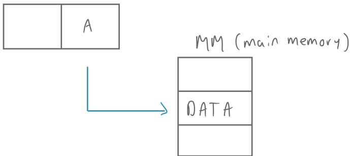
The address field A in the instruction **directly specifies** the memory location where the data is stored
